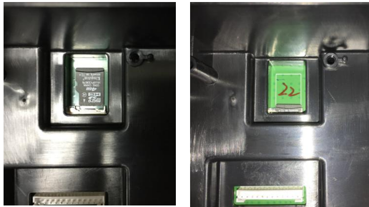
Figure 2-5 Sliding an SD Card into the SD Socket (left); SD Card Installed (right)
